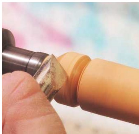
▲ Pic.29 The bead is turned next to the drive centre. The 10mm skew is used, this tool allowing a good finish and only a little of the top to be finished by hand
